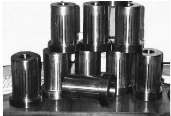
Fig. 4. Blanket flexible support cartridges (RF), developed/tested in the blanket module large project.
